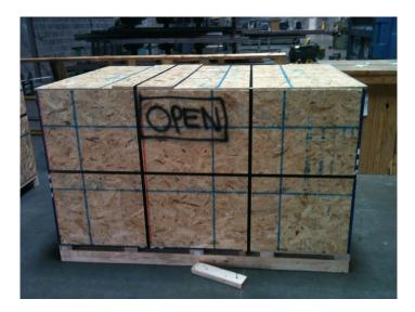
2.2 Cut and remove banding and unscrew the side marked (open this side) using a Phillips #2 screwdriver or a screw gun.
